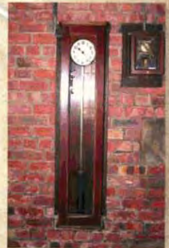
The Master Clock which regulated the whole system plus the Striking and Chiming timer which set in motion the striking mechanism.
